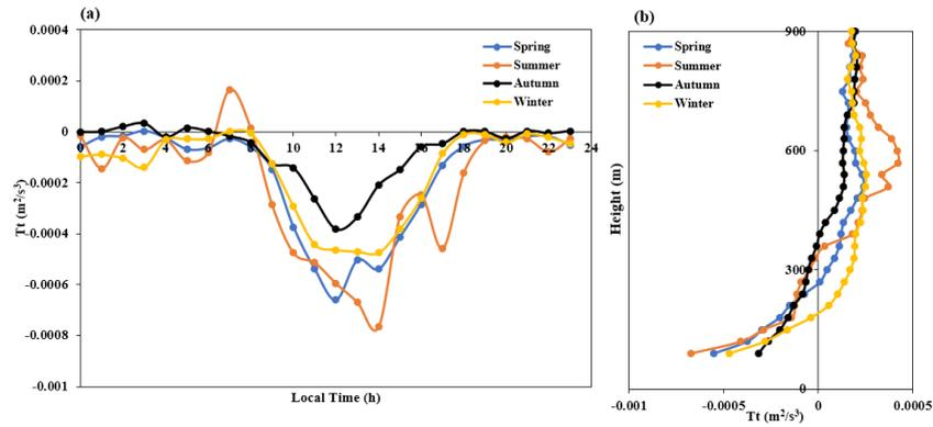
275 **Figure 13.** Time-varying curves of the turbulent transport term in the different seasons at a height of 120 m (a), as well as the distribution profile with height at 13:00 for each season (b).
