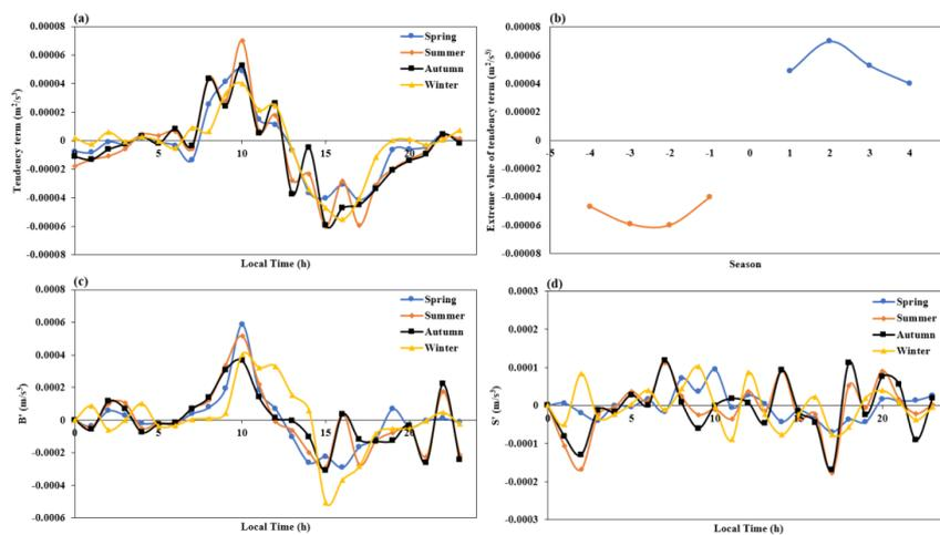
200 **Figure 6.** Time variation curve (a) and corresponding extreme value variations (b) of the TKE tendency term in different seasons at a height of 120 m, as well as the corresponding change rate of the buoyancy generation term (c) and shear generation term (d).
