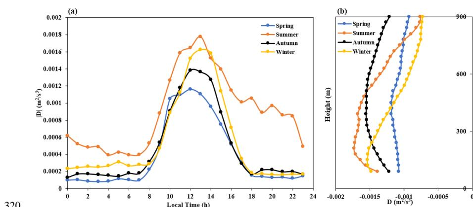
320 **Figure 17.** Time-varying curves of the dissipation rate in the different seasons at a height of 120 m (a), as well as the distribution profile as a function of height at 13:00 local time (b).
