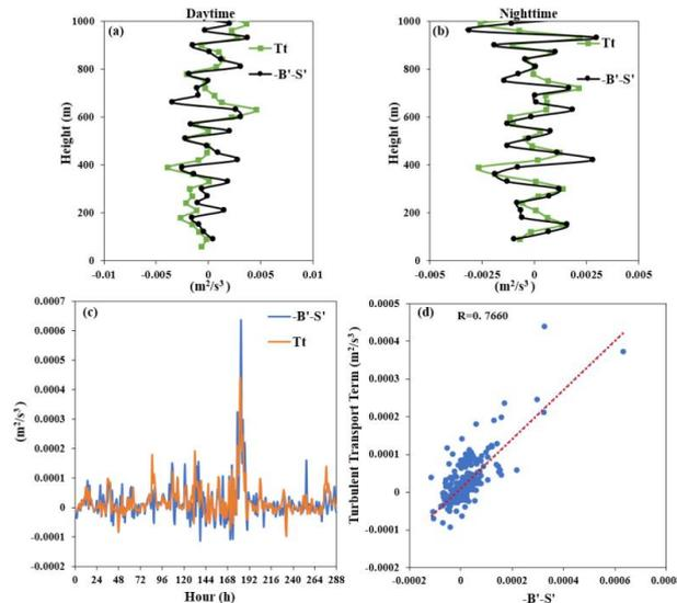
285 **Figure 14.** Variation curves of the spatial derivatives of the turbulent transport term, buoyancy generation term, and shear generation term during the daytime (a), at night (b), at a height of 120 m over the whole year (c), and the corresponding correlation (d).
