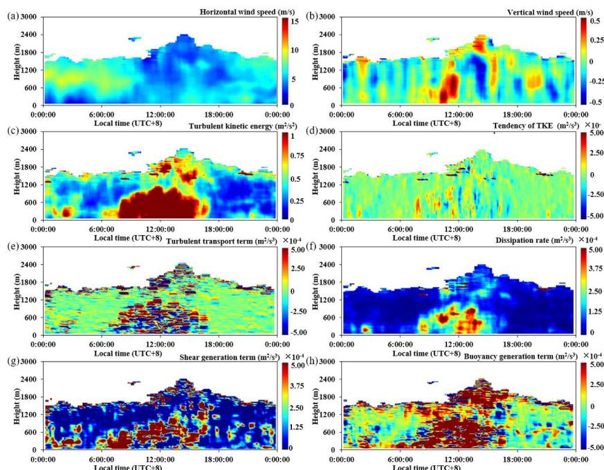
150 **Figure 2.** Temporal and spatial distributions of the horizontal wind speed (a), vertical wind speed (b), TKE (c), tendency term (d), turbulent transport term (e), dissipation rate (f), shear generation term (g), and buoyancy generation term (h) on September 21, 2022.
