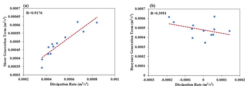
305 **Figure 16.** Correlation between the dissipation rate and the shear generation term (a) and buoyancy generation term (b) during the night.
