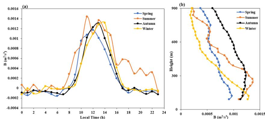
**Figure 8.** Time-varying curves of the buoyancy generation term in the different seasons at a height of 120 m (a), as well as the distribution profile with height at 13:00 local time for each season (b).
